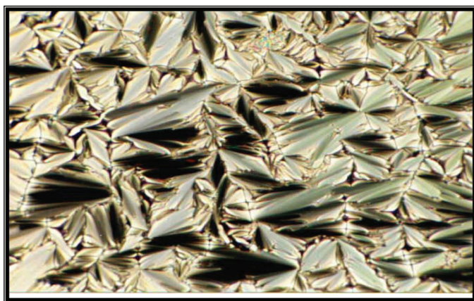
FIGURE 4 Polarizing micrograph of the focal conic texture of the smectic A phase ( \times 200 magnification) for the compound [X]_3 at 125^\circ\text{C} on cooling.
